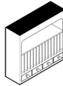
WCPR3. Plate rack with shelf over and spice drawers under. Space for plates 300mm high.
