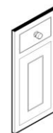
AH4. Integrated appliance door with dummy drawer in a frame. (full size)
