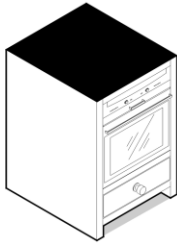
OH1. Base cabinet, built-in single oven housing, pull down tray space below.
