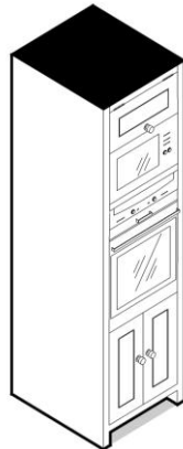
OH7. Tall built-in single oven and micro/coffee/steam oven housing. 1 top hinged door above, 2 doors below.
